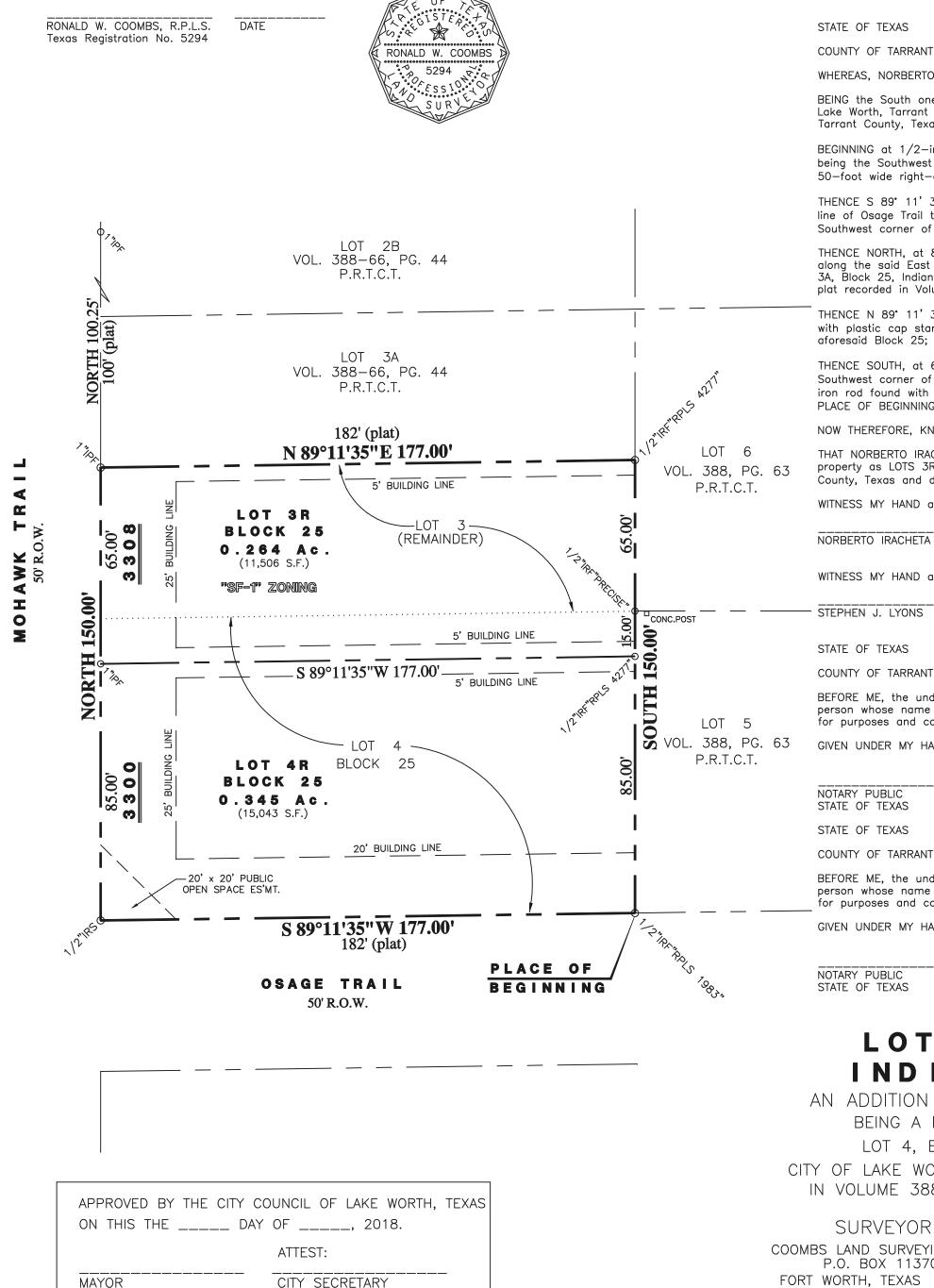
IRF DENOTES IRON ROD FOUND IRS DENOTES IRON ROD SET W/ORANGE PLASTIC CAP STAMPED "R. W. COOMBS RPLS 5294" C.M. DENOTES CONTROLLING MONUMENT BASIS OF BEARINGS: EAST RIGHT-OF-WAY LINE ( MOHAWK TRAIL AS SHOWN ON PLAT RECORDED IN VOL. 388, PG. 63, P.R.T.C.T.
